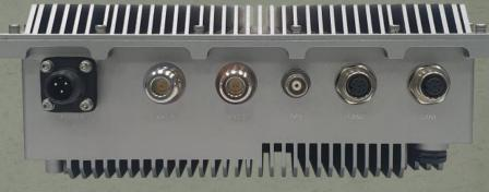
4.5 GHz 3 Watts MIMO Radio
